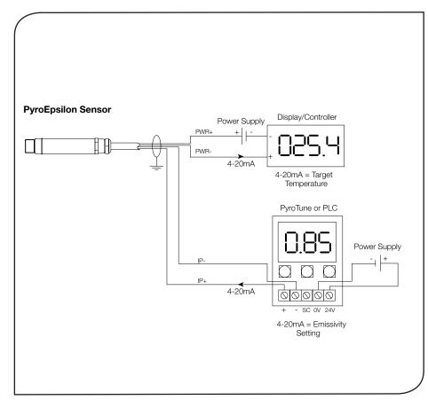
The PyroEpsilon Series is a range of high quality, low cost, compact sensors which measure the temperature of inaccessible or moving objects and materials. They measure temperatures from -20°C to 500°C, accurately and consistently, with an outstanding response time of 240 ms.
